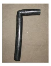
Attach the long end of the rubber hose to the end of the other 90° elbow. (Reference photo below for orientation of hose with connectors) Install the intake air temperature sensor and rubber grommet from the air intake duct resonator into the <sup>3</sup>/<sub>4</sub>" diameter hole located in the neck of the performance air box lid.
